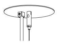
Mounting Option Power 1A Octagon Box (By Others) Installed in drywall, wood or concrete ceiling
