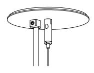
Mounting Option Power 3A 65mm Diameter Box (By Others) Installed in drywall, wood or concrete ceiling
